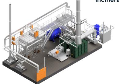
Our solution for ultra-low emissions, these incinerators are integrated with dry gas scrubbing, flue gas filtration, and heat recovery. These plants comply with South African and EU emission regulations.
